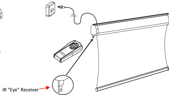
**4. IR Remote Control:** The Infrared functions by direct line of sight contact with a beam range of 30 feet.
