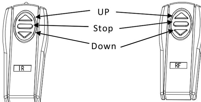
**5. RF Remote Control: (Not Included)** The radio waves eliminate the need for a direct line of sight with a range of 150 feet.
