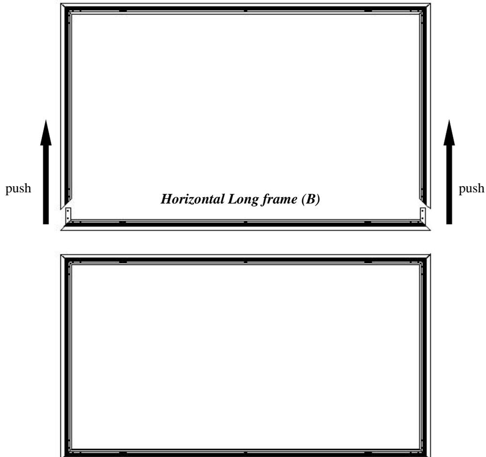
8. Make sure all four corners are properly in place to form a perfect square. Then fasten the four angles with the **M5x15 Screws (H)**.
