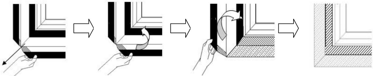
1) Stretch the screen material in the direction of the arrowhead.
