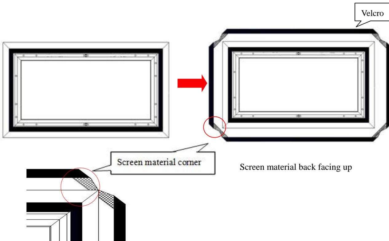
3. After all of the corners of the frame have been properly aligned, attach the material to the frame in the following order A→B→C→D (see instructions below for details).
