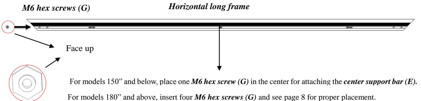
5. Insert the *elbow joint* (A) into each end of the *horizontal frames* (B) as shown below.
