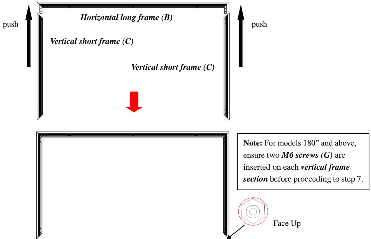
7. Join the remaining *horizontal long frame (B)* with the frame built in the previous steps as shown below.
